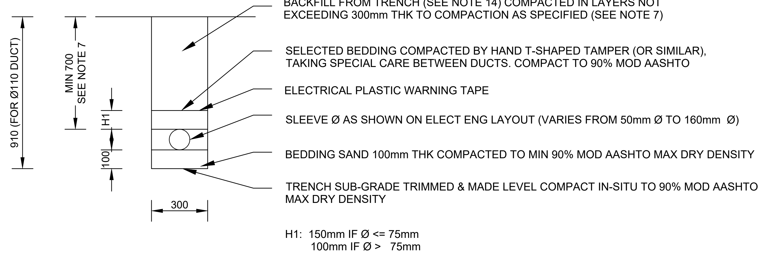
DETAIL CT-01: SINGLE PIPE N.T.S.
